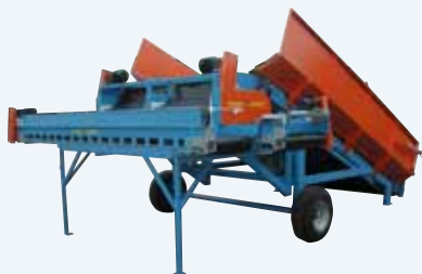
Intake with bufferhoppers and boxfillers.
